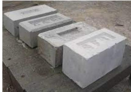
**Fig.3 Fly Ash Brick**
