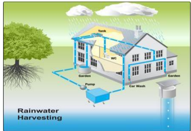
Fig.3:- Rainwater Harvesting System
