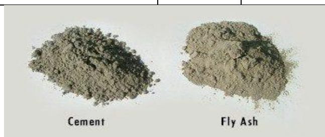
Figure 3 Cement and Fly ash
